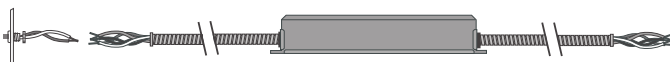
L30-DC-CEC: Dual flex conduit on each end, with test switch and plate
